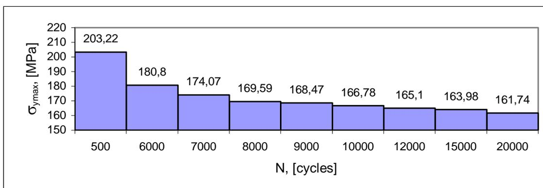
Fig.1 Loading fatigue block  $\sigma_{y\max}$  – N
