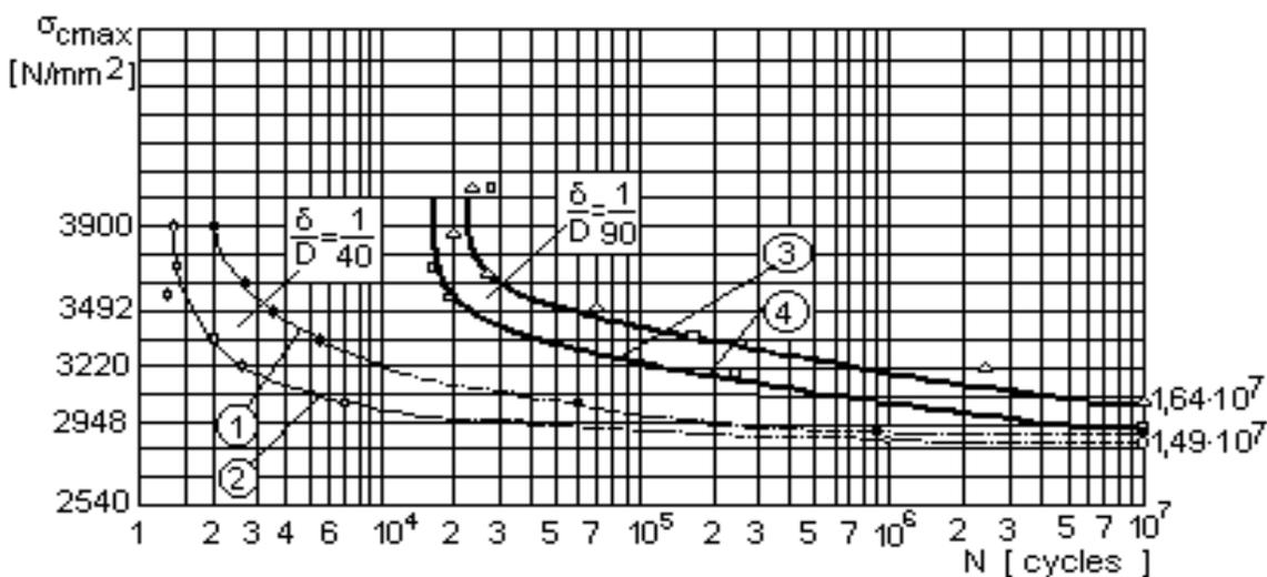
**Fig.2** The lifetime variation for the tested wires on the [NB] testing machine, in function of the contact compression stress
