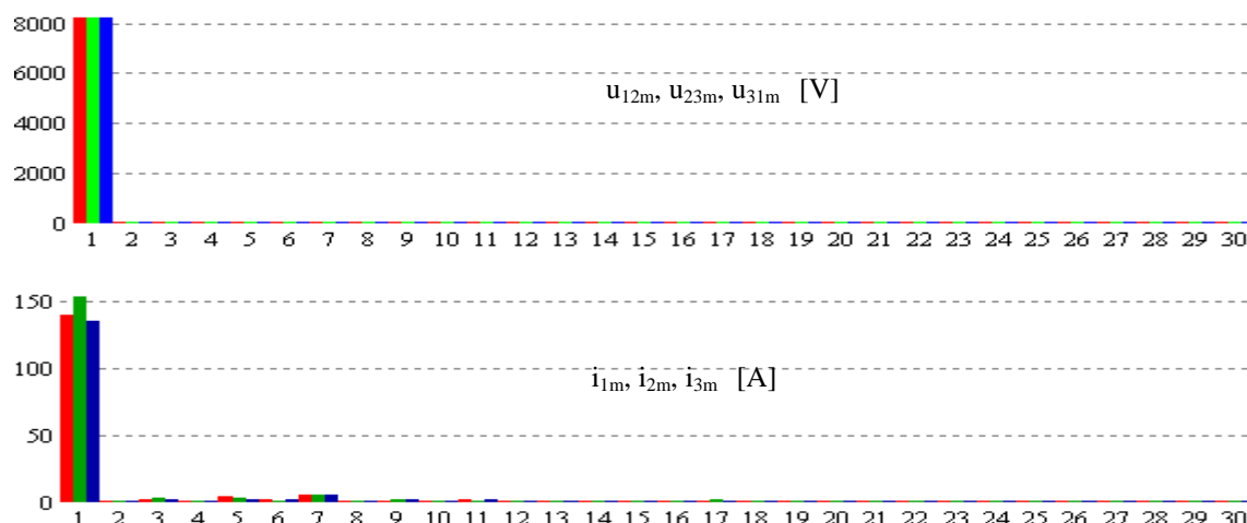
Fig. 12 The harmonic spectra of the signals acquired on the mean voltage line at the end of the cast-iron's melting process.
