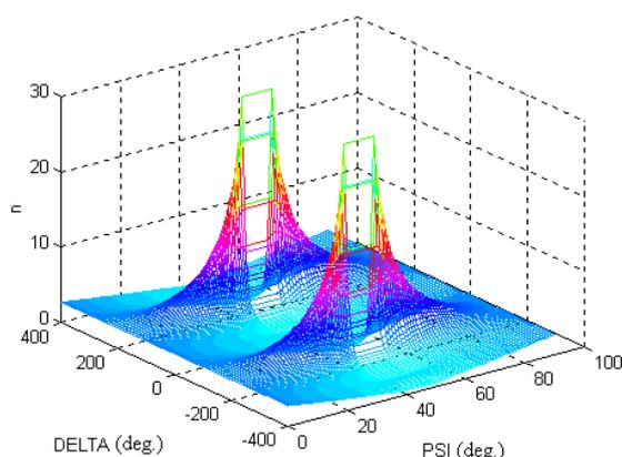
Fig. 1 Dependence of optical constants  $\bar{n}$  on ellipsometrical magnitudes  $\Delta$  and  $\Psi$ .
