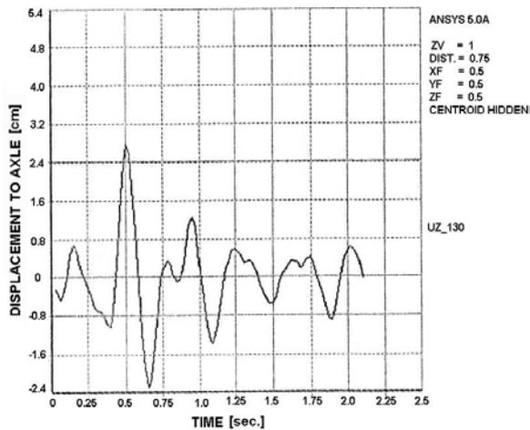
Figure 4 - The wheel axle displacement (Disk harrow GD 3.2 during the transport)
