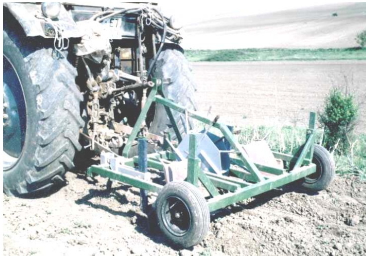
FIGURE 13. A complex machinery coupled to tractor tk-80 and an equipment for inter-row erosion control tillage along the slope.
