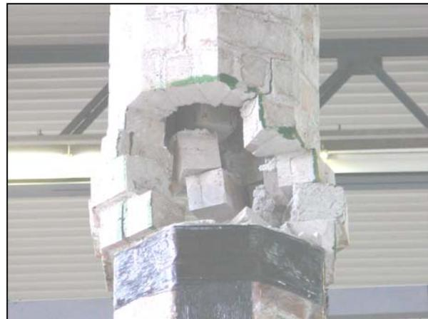
**Figure 6.** Collapse of the upper part of the minaret
