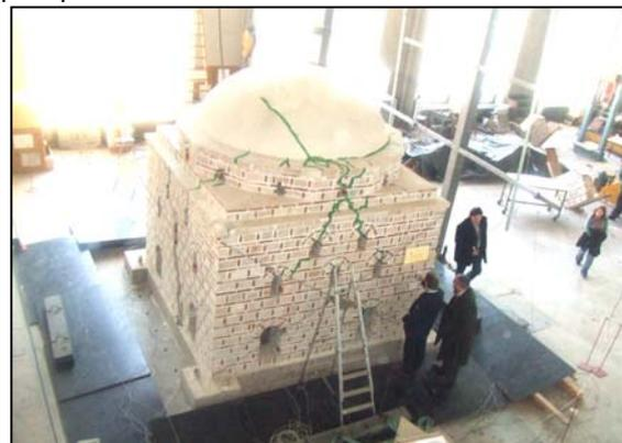
**Figure 7.** Damaged model after phase 2 testing
