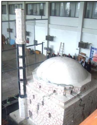
**Figure 5.** Repaired model and strengthened minaret after phase 1 testing
