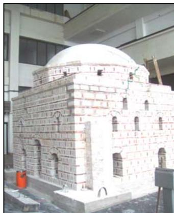
**Figure 11.** Re-built part of the model after removal of the minaret
