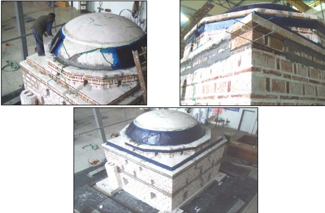
**Figure 12.** Details of strengthening and strengthened model ready for testing, phase 3
