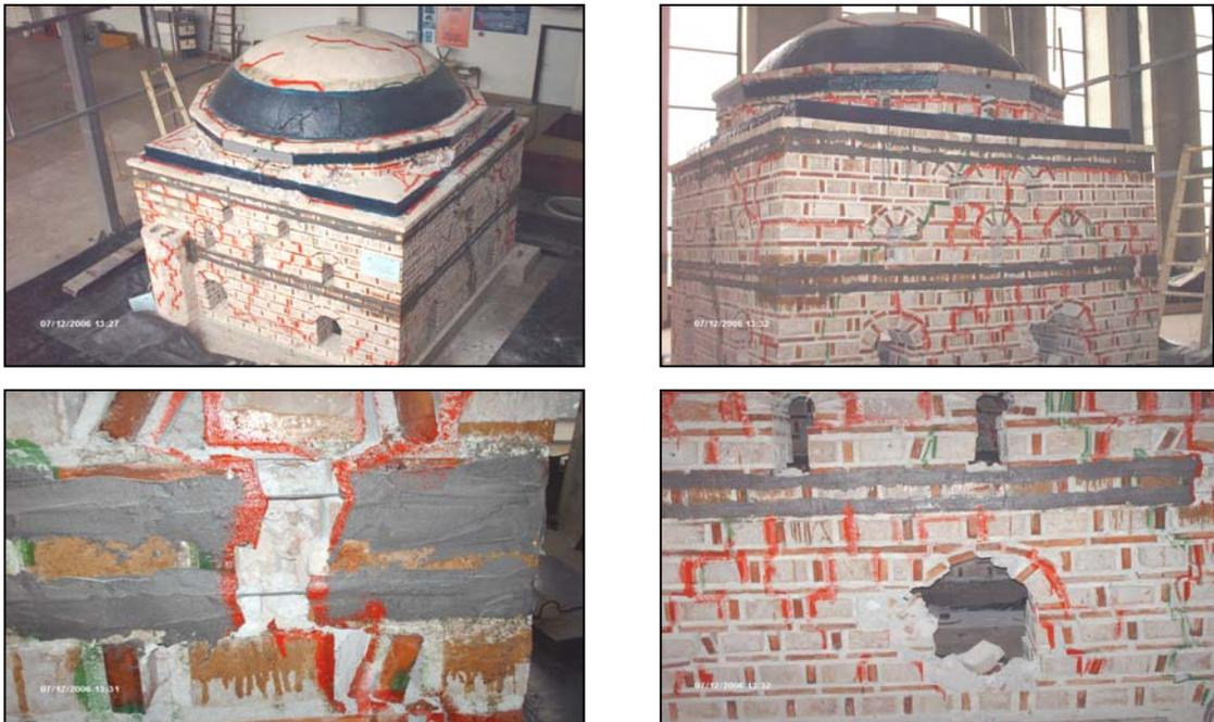
**Figure 13.** Damage of the model after phase 3 tests accomplishment
