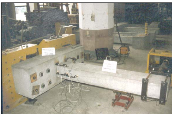
Figure 1. Disposition of the beam and column models and the equipment during quasi-static tests
