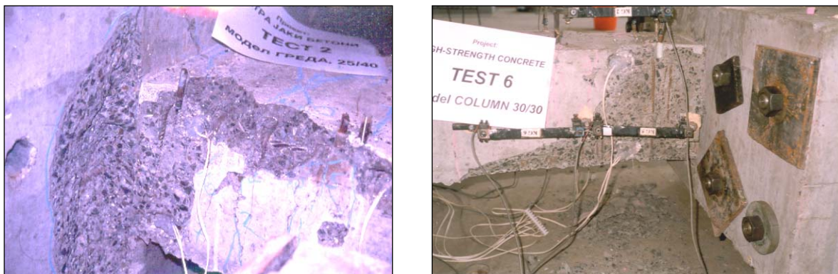
Figure 3. Experimental investigations of beam and column models, (damage observation)
