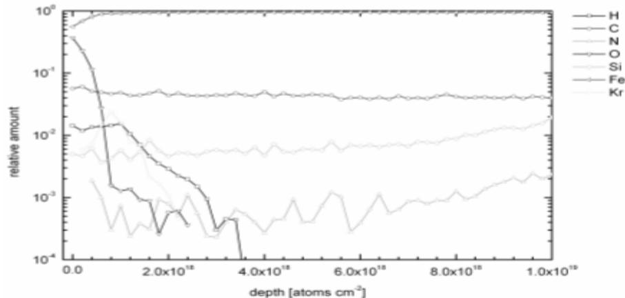
Figure 13. Results ERDA analysis for sample – Kr<sup>8+</sup>
