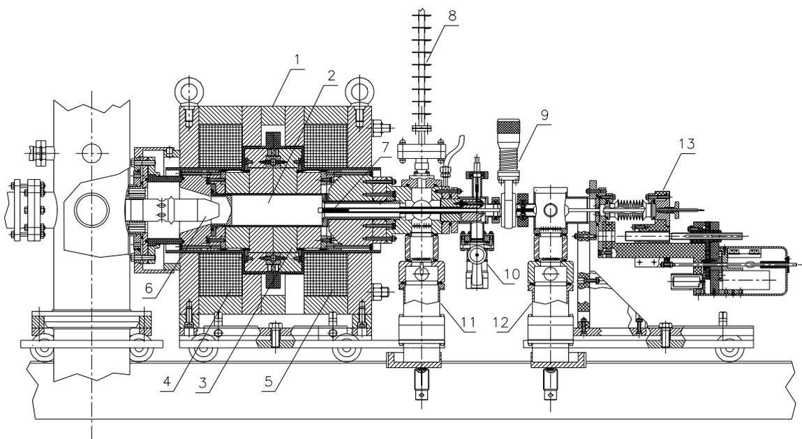
**Figure 4.** ECR ion source with solid substance inlet system: 1-yoke, 2-plasma chamber, 3-hexapole, 4-extraction stage coil, 5-injection stage coil, 6-extraction electrode, 7-minioven installed inside the bias electrode, 8-waveguide, 9-gate valve, 10-gas dosing valve, 11 and 12-turbo- molecular pumps, 13-minioven positioning system
