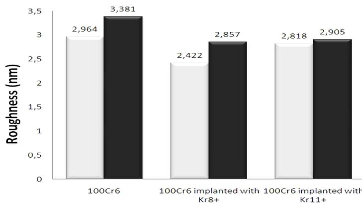
**Figure 9.** Surface roughness measurements for 100Cr6 steel (minimum and maximum measured values)
