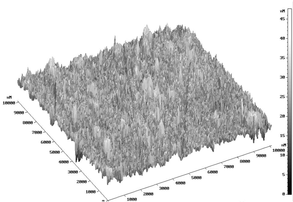
Figure 10. AFM image 100Cr6 steel implanted with Kr<sup>11+</sup>
