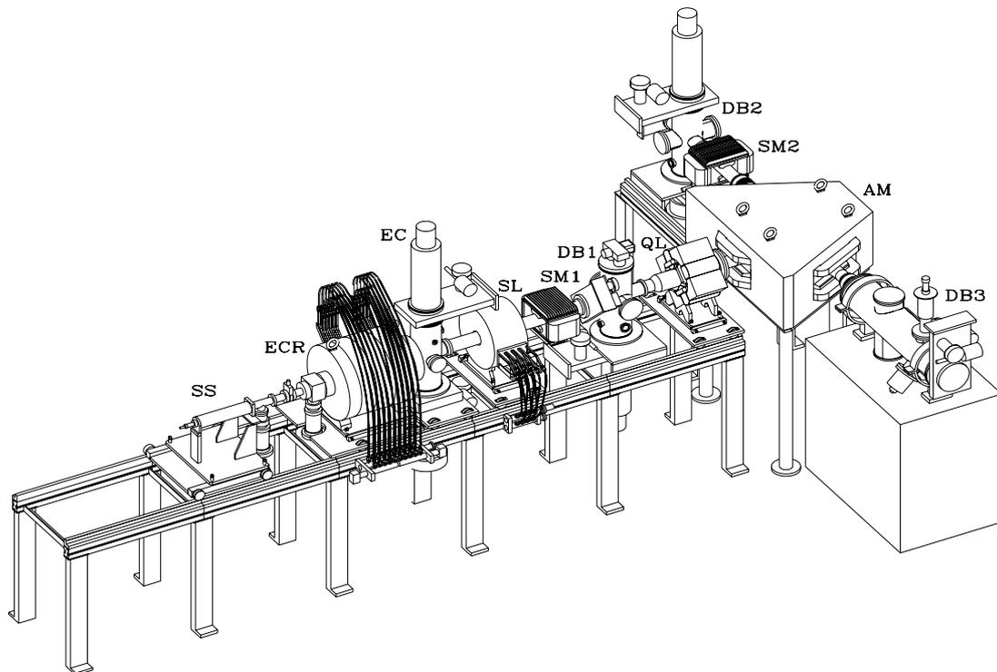
**Figure 3.** mVINIS Ion Source as a complete heavy ion injector.
