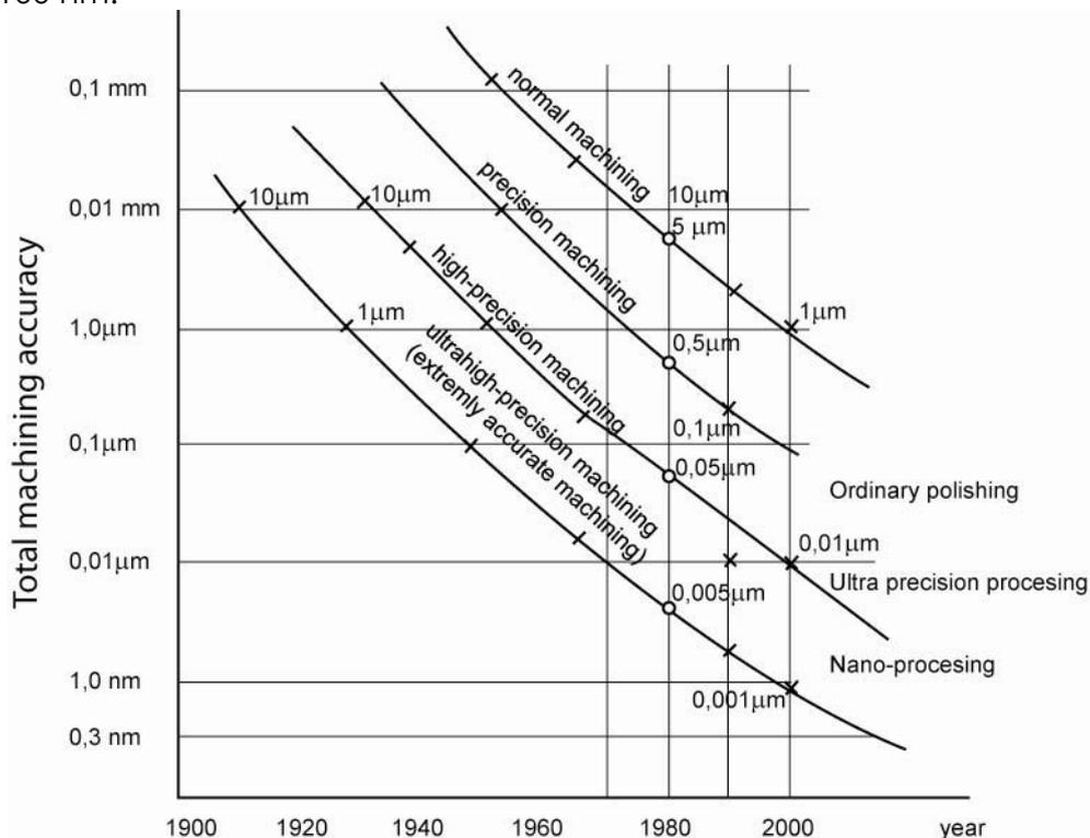
Figure 1. Trends in precision machining by Taniguchi [1]
