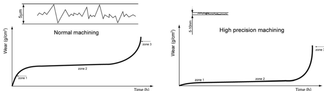
Figure 2. Tools wear during normal and high precision machining
