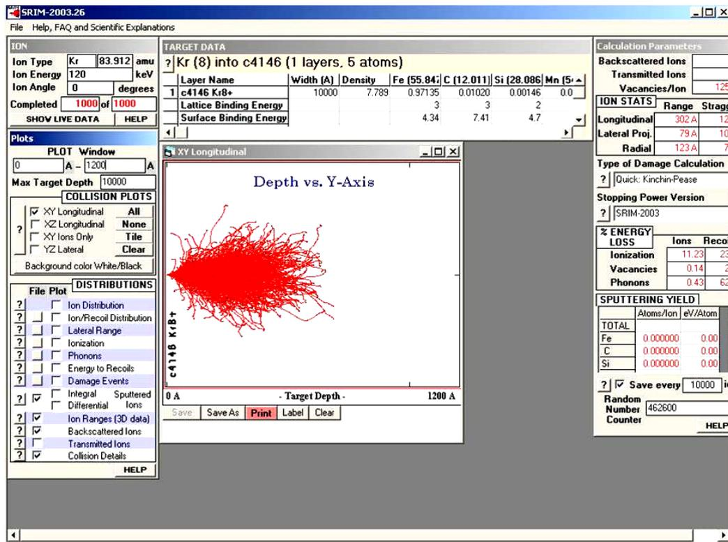
Figure 6. SRIM simulation of Kr<sup>8+</sup> ions into 100Cr6 steel
