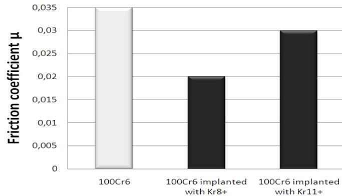
**Figure 8.** Friction coefficients for  $F=10N$
