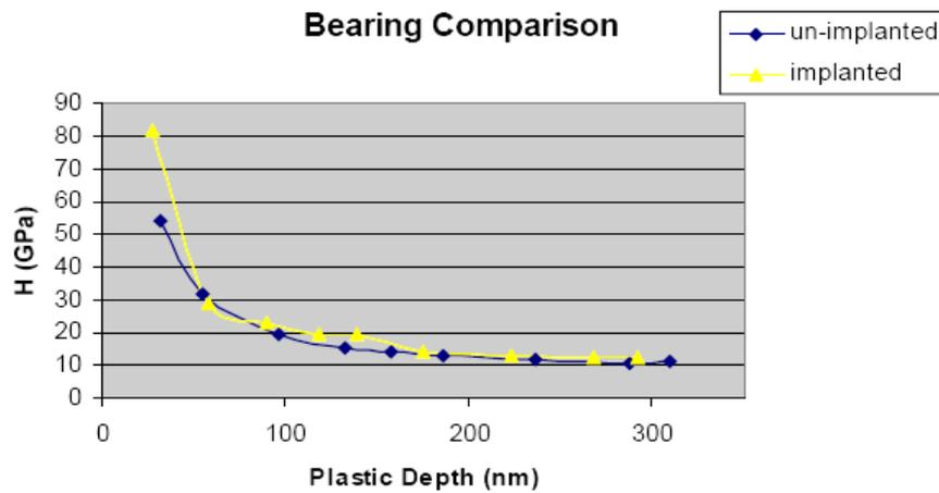
Figure 11. Kr<sup>11+</sup> implanted 100 Cr 6 steel - comparison regarding hardness
