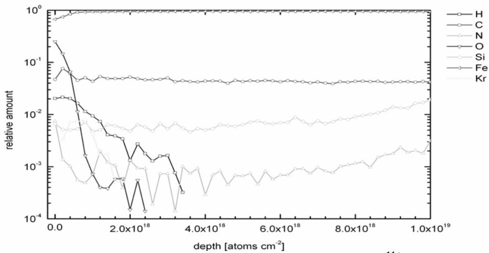
Figure 12. Results ERDA analysis for sample – Kr<sup>11+</sup>
