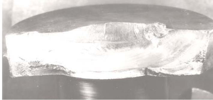
Fig. 5. Fracture area of the crank shaft at the first break-down (analysis ZTS MATEC, 27.1.2000)
