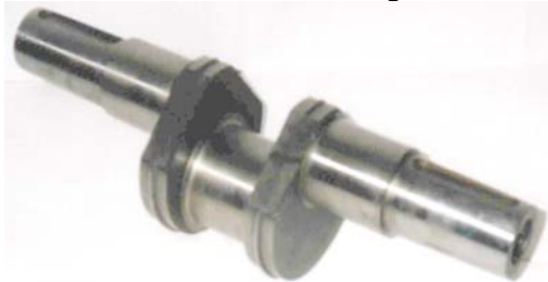
Fig. 3 Crank Shaft of the BL 50-250 press
