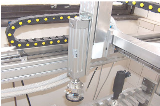
Figure 2A. Portal 3-axes Smc – robot
