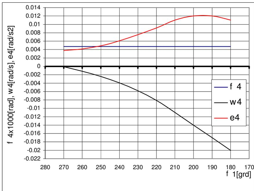
Figure 4. Variation of to position angle, angular velocity and angular acceleration for big driving rod 4 depending on angle f1
