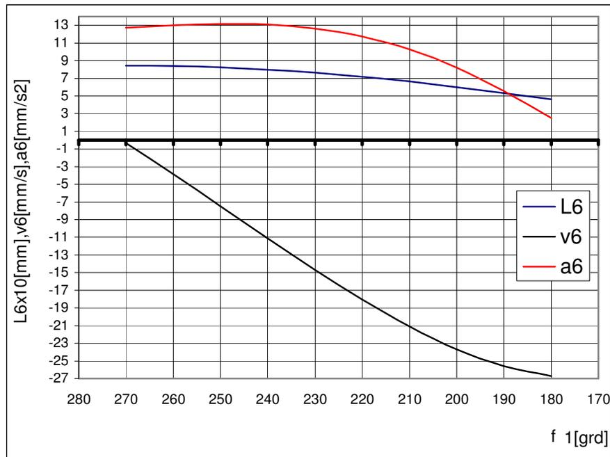
Figure 5. Variation of movement, linear velocity and linear acceleration for superior slider 6 depending on  $f_1$
