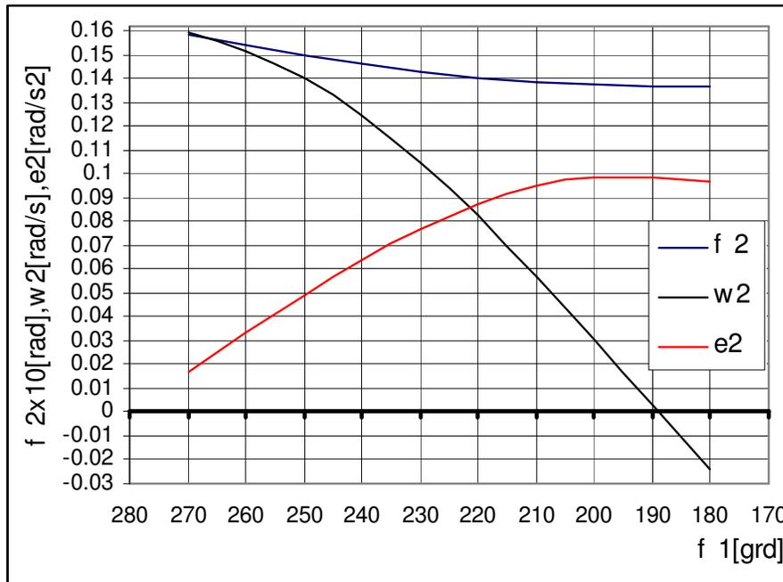
Figure 2. Variation of to position angle, angular velocity and angular acceleration for small driving rod 2 depending on angle f1
