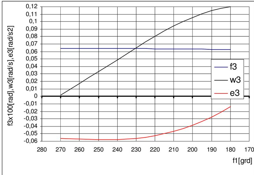
Figure 3. Variation of to position angle, angular velocity and angular acceleration for higher arm 3 depending on angle f1
