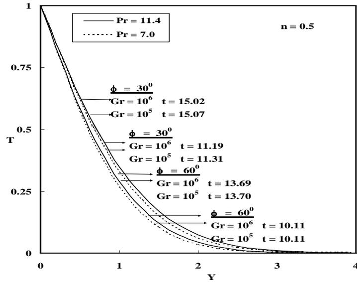
Fig.5 Steady state temperature profiles at  $X=1.0$  for different Gr and  $\phi$
