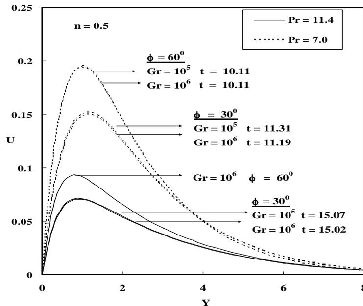
Fig.4 Steady state velocity profiles at X=1.0 for different Gr and  $\phi$
