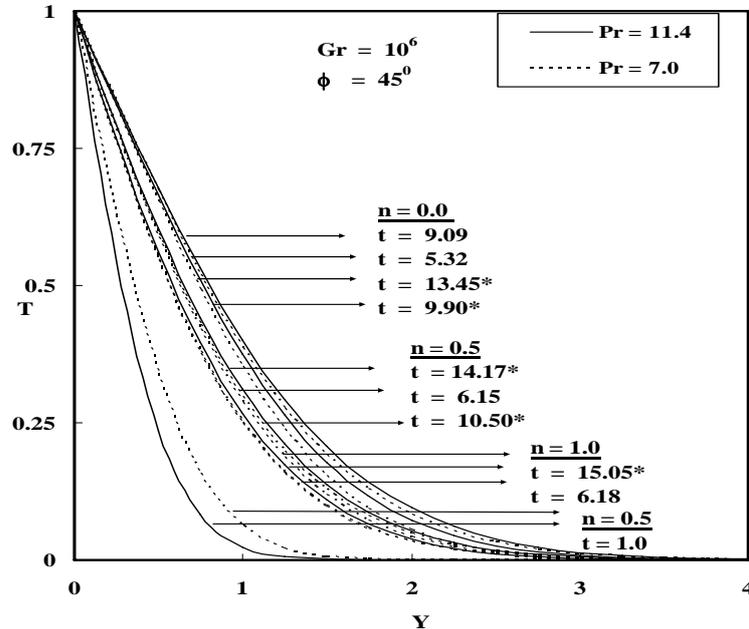
Fig.3 Transient temperature profiles at X=1.0 for different n (\* - steady state)
