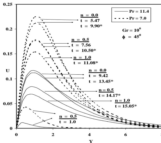
Fig.2 Transient velocity profiles at  $X=1.0$  for different  $n$  (\* - steady state)
