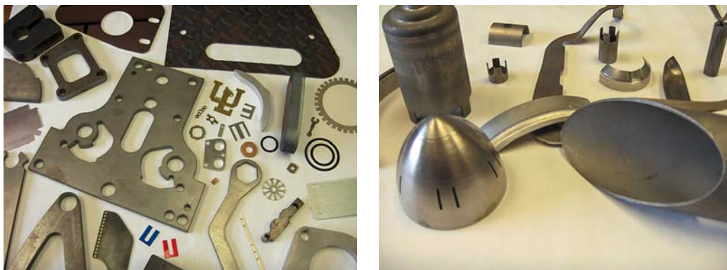
FIGURE 1. EXAMPLE OF PARTS MADE USING 2D AND 3D LASER
