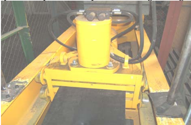
FIGURE 1. Testing board with a hydraulic system
