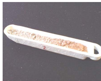
Figure 4. Sample melted at 1200°C
