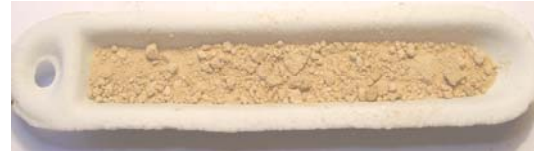
Figure 7. Sample melted at 900°C
