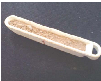
Figure 3. Sample melted at 900°C
