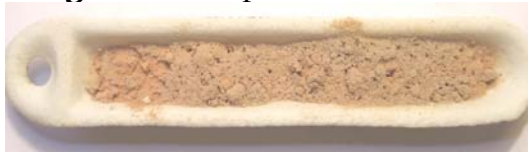
Figure 8. Sample melted at 1000°C
