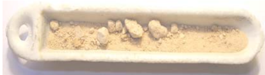
Figure 6. Sample melted at 800°C
