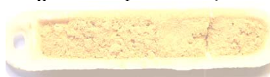
Figure 9. Sample melted at 1100°C
