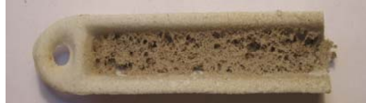
Figure 10. Sample melted at 1230°C
