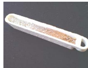
Figure 5. Sample melted at 1350°C
