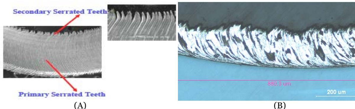
Figure 2. Schematic of the chip: (A) SEM top view of the chip with the serrated element (B) length wise sectional view under optical microscope
