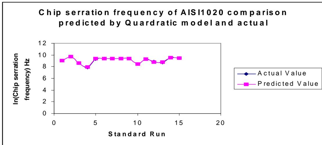
Figure 4. Chip Serration Frequency contours of experimental and quadratic CCD predicted values
