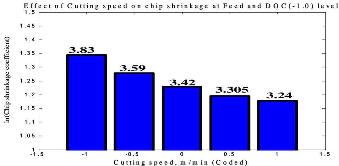
Figure: 6 Effect of Cutting Speed on chip shrinkage coefficient
