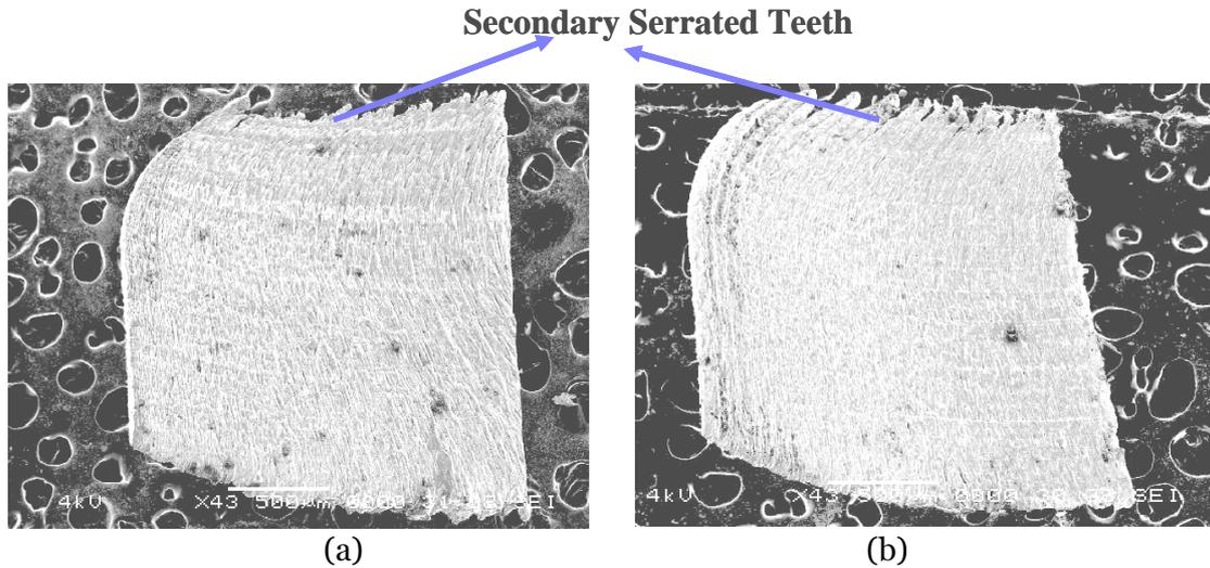
Figure 3. Sample SEM View of the AISI1020 chip at different cutting speed (a) CS 120m/min (b) CS 300 m/min with same Depth of Cut 1.59mm, feed: 0.089mm/tooth
