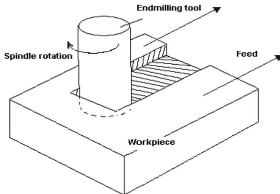
Figure 1 Experimental set up for end milling
