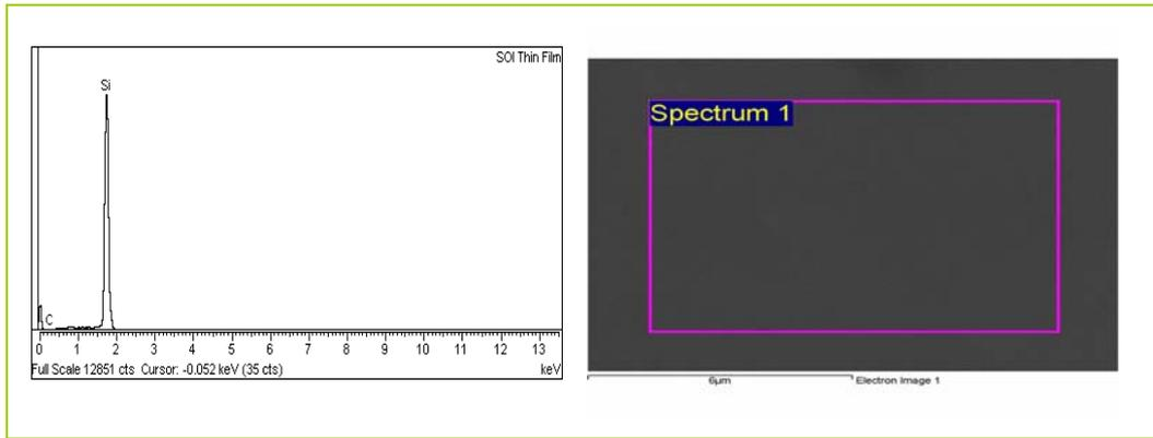
**Figure 1.** EDX Picture of Thin Film SOI
