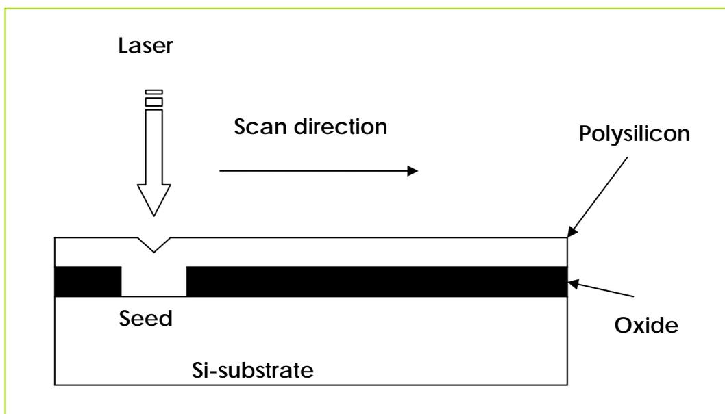
**Figure 3.** Process flows for Zone –Melting and Recrystallization
