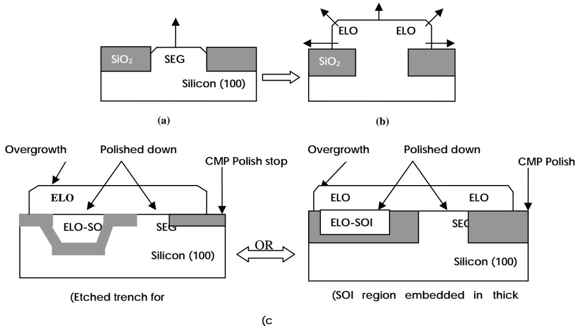
**Figure 2.** Cross sections of (a) SEG growth, (b) ELO growth, and (c) SEG/ELO with CMP planarization forming completely isolated SOI “well”.
