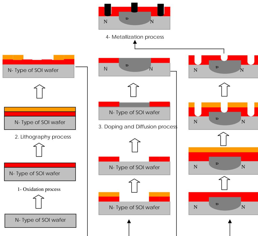
**Figure 4.** Subsequent of the steps fabrication process
