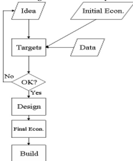
**FIGURE 1.** Schematic workflow of Pinch Approach
