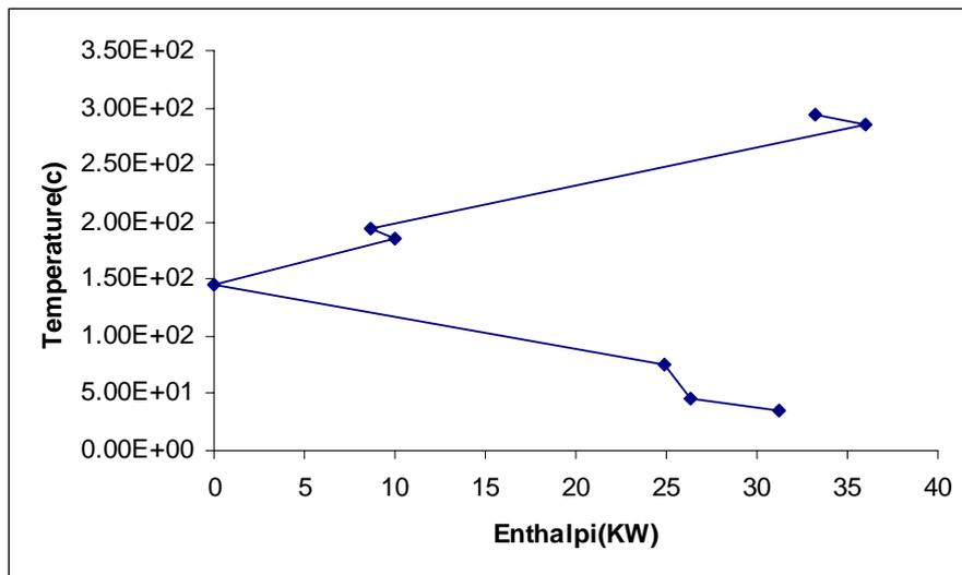
**FIGURE 6.** Grand Composite curve at  $DT_{min, optimum} = 11^{\circ}C$
