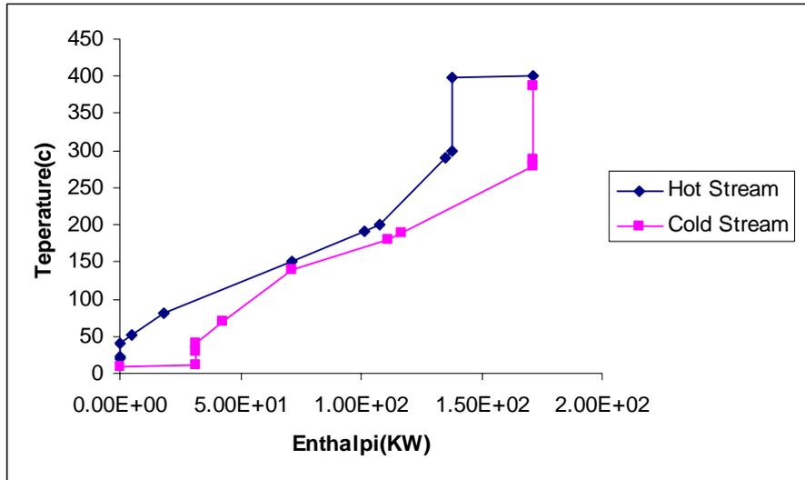
**FIGURE 5.** Balanced Composite curve at  $DT_{min, optimum} = 11^{\circ}C$
