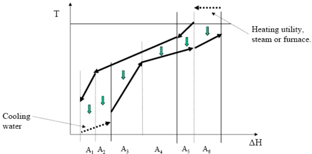
**Figure 2.** Vertical heat transfer
