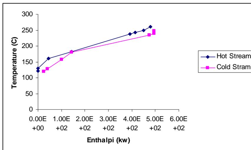
**FIGURE 8.** Composite curve at  $DT_{\min, \text{ optimum}} = 2\text{ }^{\circ}\text{C}$
