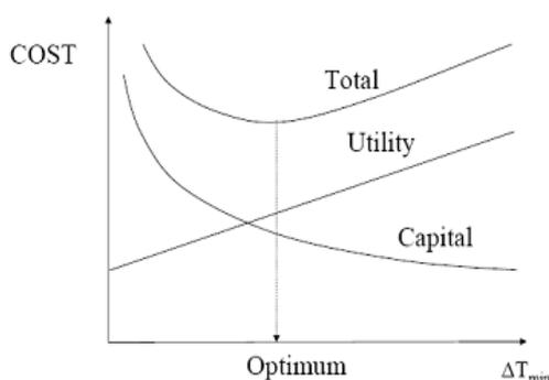
**FIGURE 4.** The trade-off between energy (utility) and capital cost to give the optimum  $DT_{min}$
