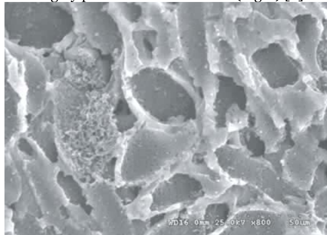
FIGURE 1. Electron microscope photograph of activated carbon pores
