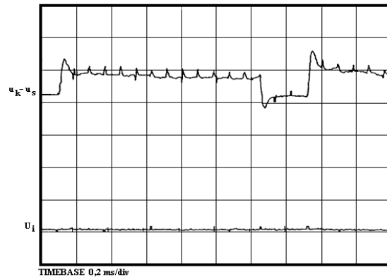
Figure 9. The voltage at the motor terminals and the output voltage of the analog memory - detail
