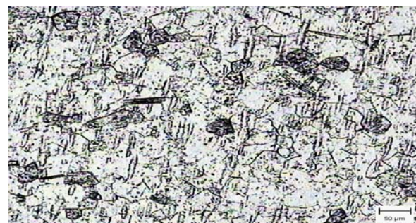
Figure 2. Titanium alloy substrate BM (cupric solution, 100 x)
