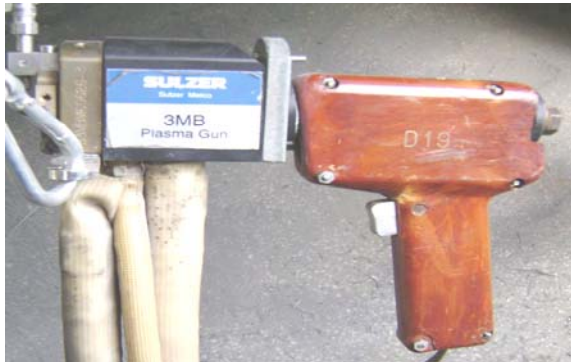
Figure 3 The thermal spraying gun 3MB of the plasma thermal spraying installation
