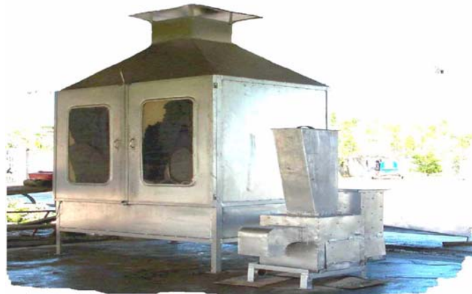
Fig. 4 Dryer FD-50 fed with thermal energy from a cross-draft gas generator
