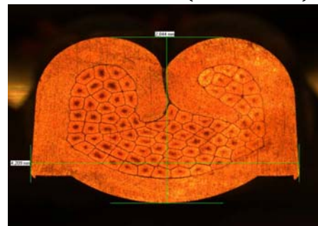
Figure 2. Section through the terminal
