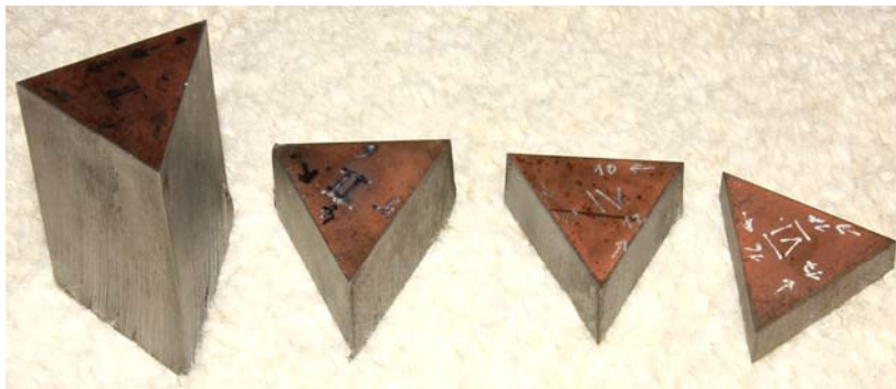
FIGURE 1. Detail of a triangular footprint shape of the samples (from the left: 40, 15, 10, 6 mm; 2 of 3 cut surfaces displayed)
