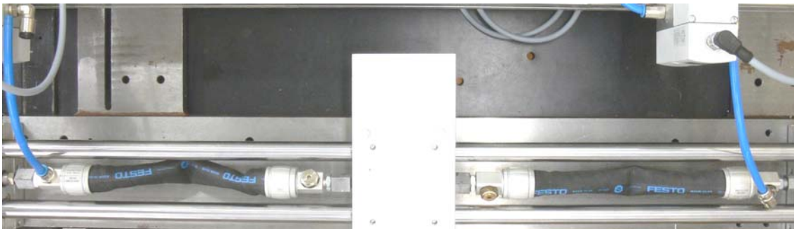
Figure 7. Mounting pam's into shorter places than their initial lengths
