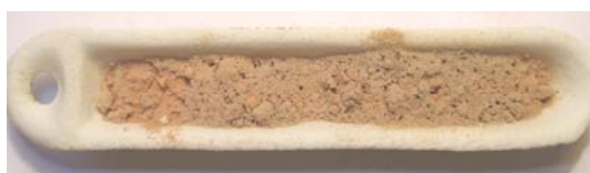
Figure 8. Sample melted at 1000°C
