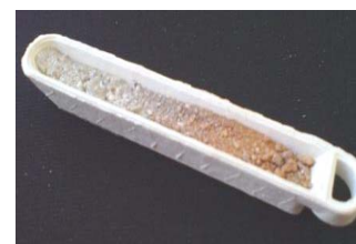
Figure 5. Sample melted at 1350°C
