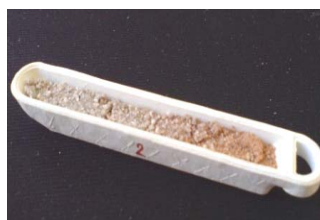
Figure 4. Sample melted at 1200°C
