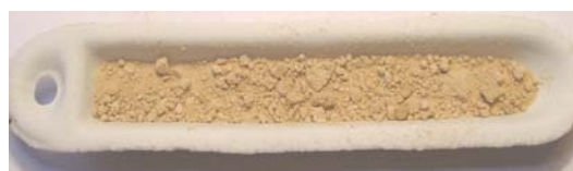
Figure 7. Sample melted at 900°C
