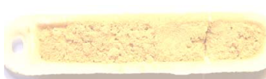
Figure 9. Sample melted at 1100°C
