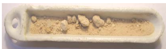
Figure 6. Sample melted at 800°C
