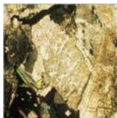
b, K-feldspar (perthititic) in granite 25x
