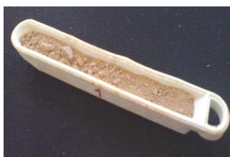
Figure 3. Sample melted at 900°C
