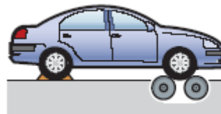
Figure 2. Car on a twin - roll dynamometer
