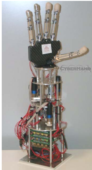
Figure 4 – The Cyberhand ( a picture of the hand assembly and kinematical structure), where: 1- palm, 2 – MP, 3 – PIP, 4 – MIP, 5 - DIP, 6 – one degree of freedom joint, 7 – two degrees of freedom joint of the thumb
