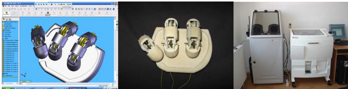
Figure 6 – The 3D model developed in SolidWorks, the resulted artificial hand and the 3D Zcorp printer used for parts fabrication
