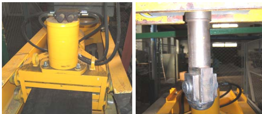
FIGURE 1. Testing board with a hydraulic system and spherical head of ram
