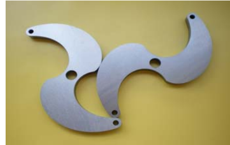
Figure 8 Involute-lantern gearing z_1 = z_2 = 2
