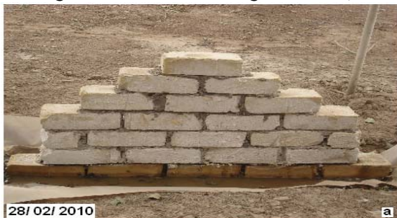
Figure 7. Walls after two weeks of soaking, a- Unprotected wall, b- Suggested wall.
