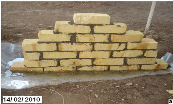
Figure 6 a. Normal testing brick wall, b- Suggested water proofing Waxy Bricks position.
