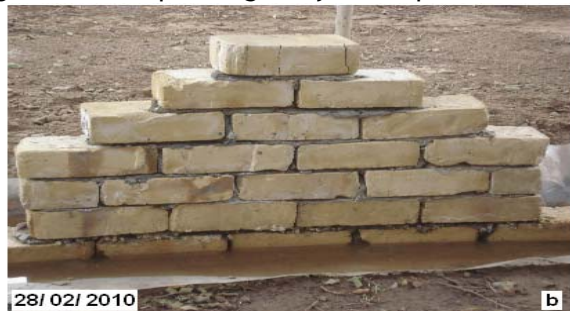
Figure 7. Walls after two weeks of soaking, a- Unprotected wall, b- Suggested wall.
