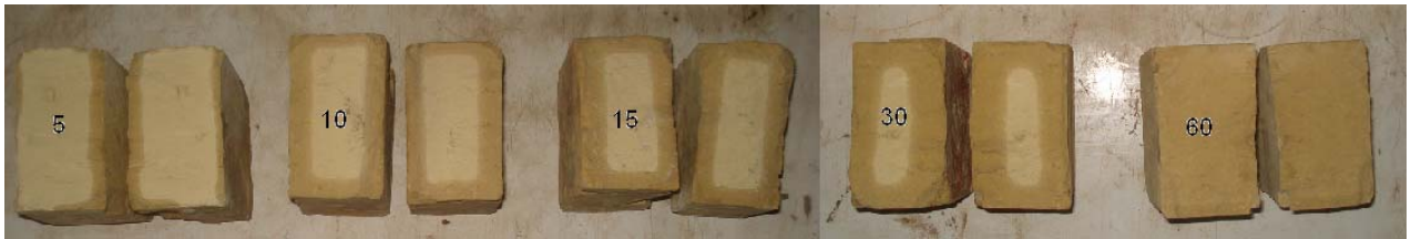
Figure 3. Wax percolations inside clay bricks with respect to time (minutes).
