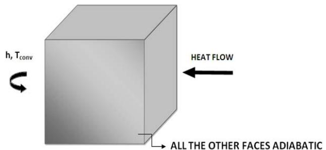
Figure 1. The Thermal boundary condition applied on the unit cell
