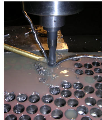
Fig.1: Drilling process of HARDOX 500 by HSS-HX drill on VR-2 drilling machine tool
