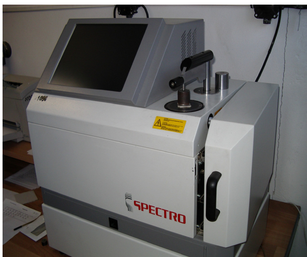
Fig.4: Overall view of the workplace spectral analysis tool material HSS-HX on the measuring device SPECTROLAB Jr-CCD
