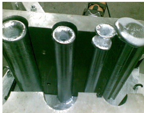
Fig. 2 Extraction of vibrated samples from the mold
