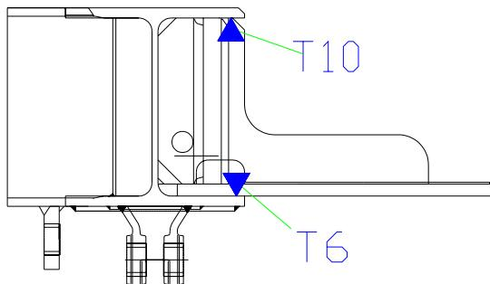
Fig. 8. Strain gauges T6 and T10
