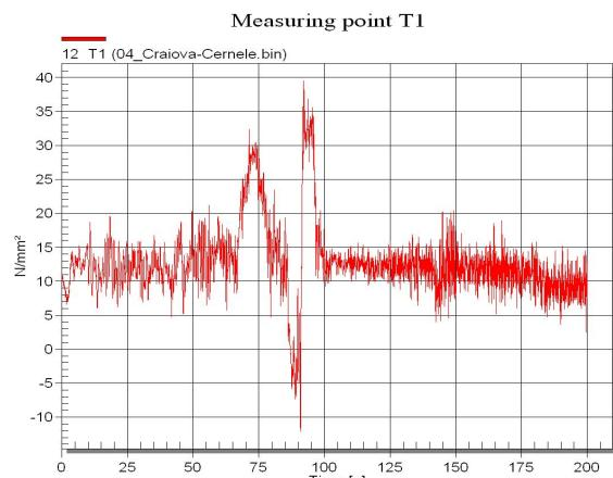
Fig. 10. T1 strain gauge stress
