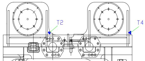
Fig. 5. Strain gauges T2 and T4
