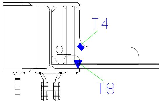
Fig. 7. Strain gauges T4 and T8
