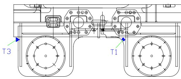
Fig. 4. Strain gauges T1 and T3
