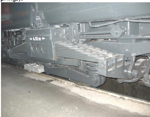
Fig. 1: Bogie with leaf spring
