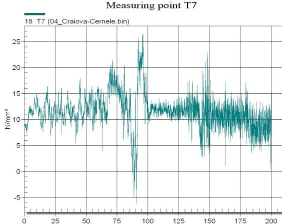
Fig. 12. T7 strain gauge stress
