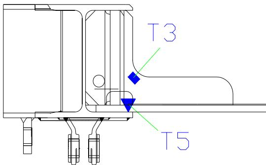
Fig. 6. Strain gauges T3 and T5
