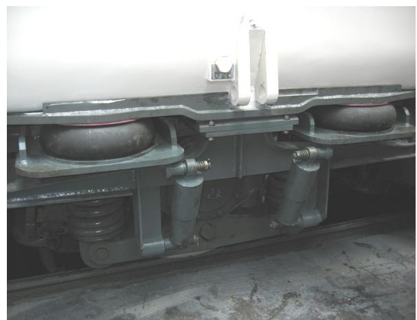
Fig. 2: Bogie with rubber spring
