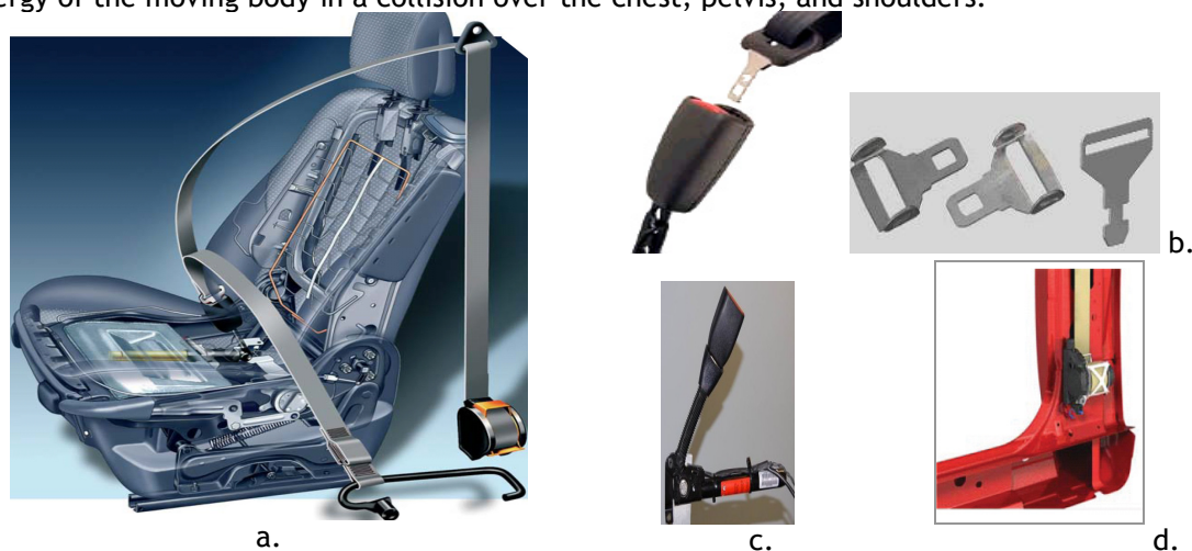
Fig.3. Standard three-point seat belt system and its components
