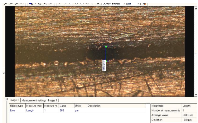
Copper alloy welding belt width: 263 μm
