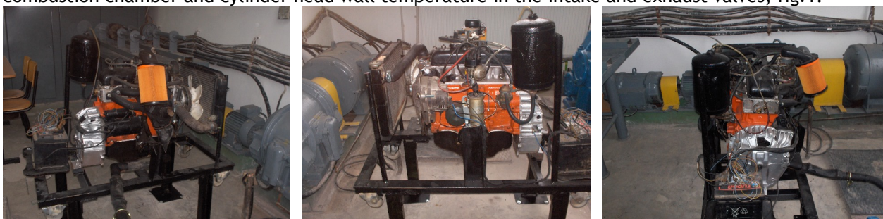
Fig.1. The experimental bench with ignition engine type Dacia
