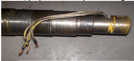
Fig.6 Thermocouples crossed through the main axis of the facility to connect their data acquisition system
