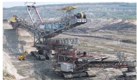
Fig. 1. Overall view of EsRc -1400 rotor excavator
