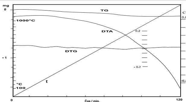
Figure 8. Derivatogram of nepheline basanite from locality Husiná
