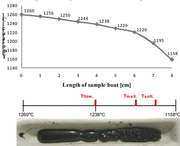
Figure 7. Temperature course of basalt sample using March furnace
