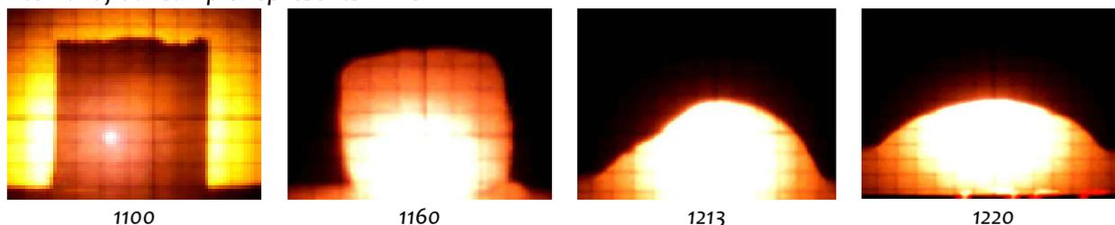
Figure 8. Basanite sample melting course on the high-temperature microscope
