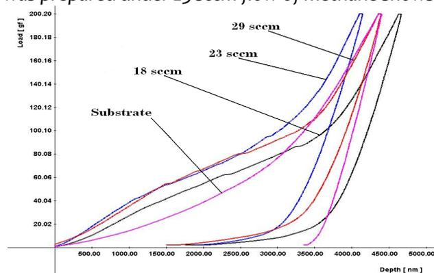
Figure 4: Record of nanoindentation test. Maximal load 200 g
