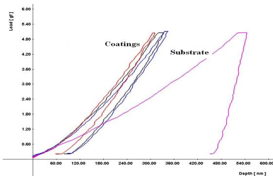
Figure 6 : Record of nanoindentation test.
