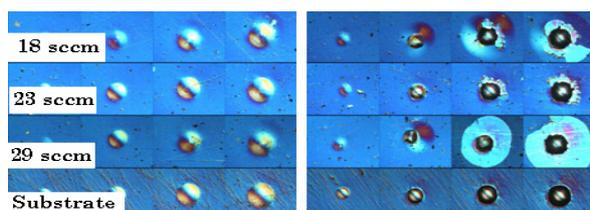
Figure 3: Morphologies of static indentation (indenter: left - 0,5 mm right - 0,2 mm)
