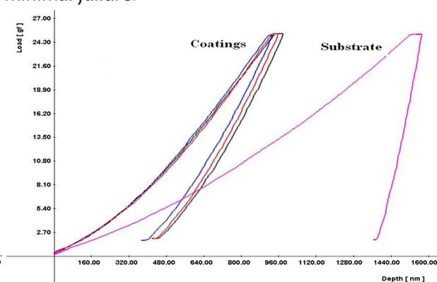
Figure 5: Record of nanoindentation test. Maximal load 25 g
