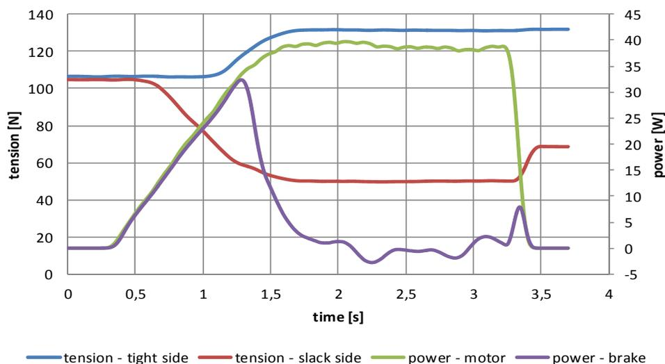
Figure 10 – Powers and tensions during the slip test
