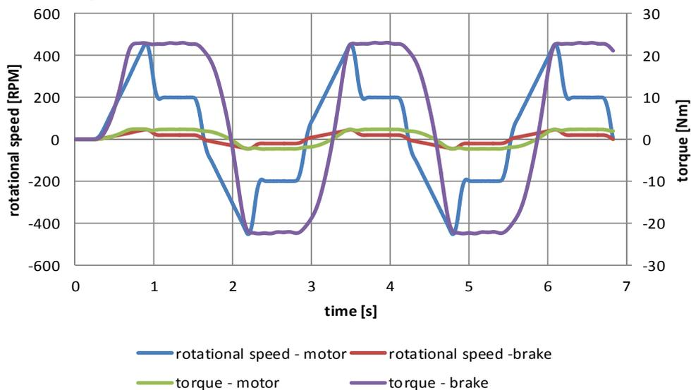
Figure 7 – Rotational speeds and torques of the motor and the brake during the combined cycle test
