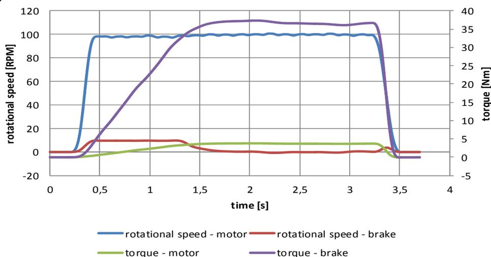
Figure 9 – Rotational speeds and torques of the motor and the brake during the slip test
