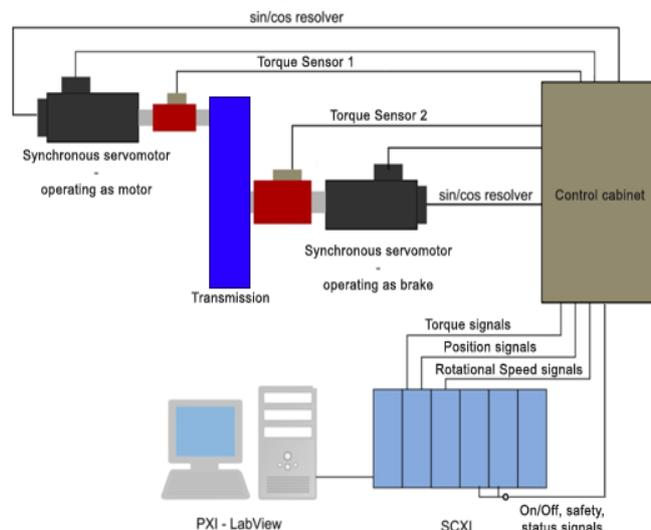
Figure 3 – Transmission test-stand – functional diagram
