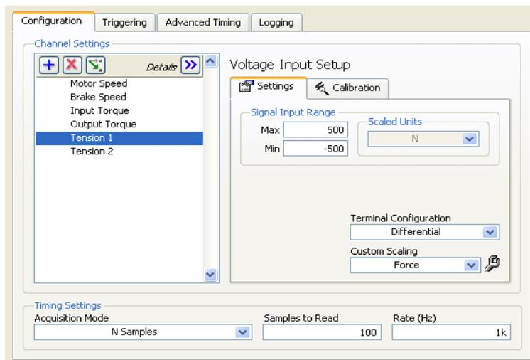
Figure 6 – Adding new channels to the task
