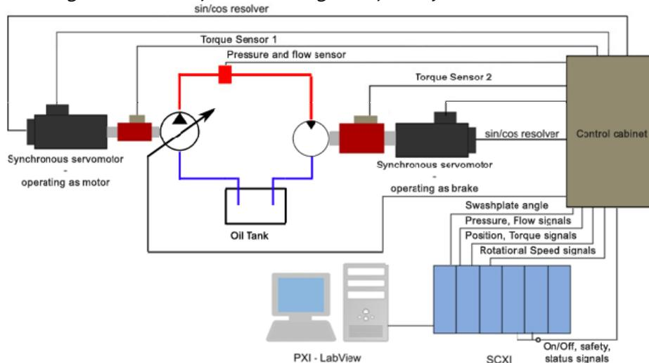
Figure 11 – Functional diagram of the hydraulic test-stand
