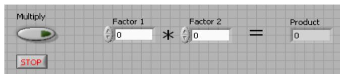
Figure 2 – Front panel of a simple multiplication program
