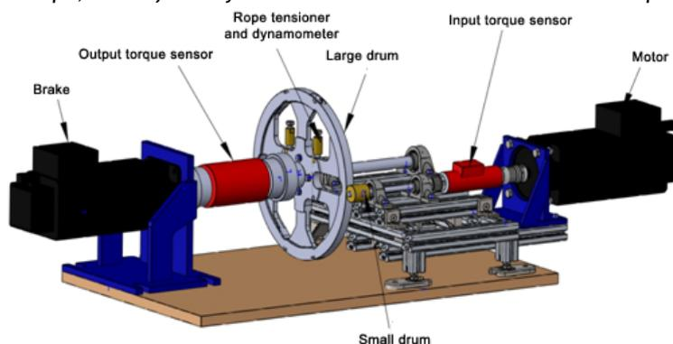
Figure 5 – Model of a transmission test-stand with the cable-drive
