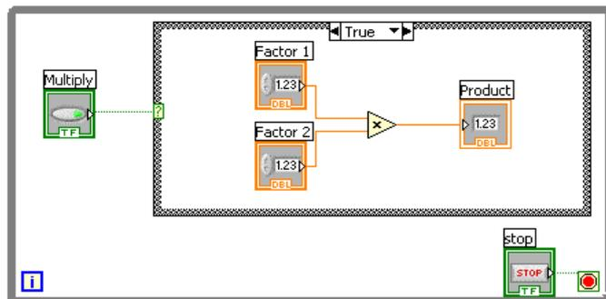
Figure 1 – Block diagram of a simple multiplication program
