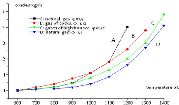
Figure 1 : Dependence of the quantity of the iron oxides, during the heating process of the non alloyed steels on the fuel, temperature and air excess coefficient,  $\varphi$
