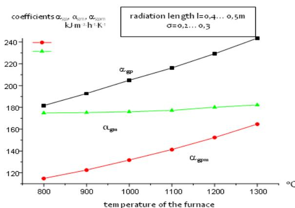
Figure 4: Variation of the coefficients  $\alpha_{gpr}$ ,  $\alpha_{gm}$  and  $\alpha_{gpm}$  depending on the temperature of the furnace, thermal radiation's length and the ratio  $\sigma$
