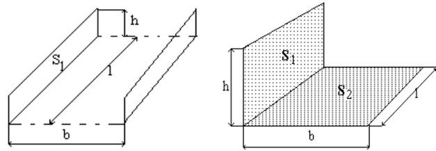
Figure 2: dimensions referring to the continuous furnaces in order to establish the coefficient  $\varphi$  [ $B=h/b$  ;  $L=l/b$ ]
