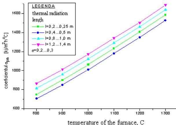
Figure 5: Variation of the coefficient  $\alpha_{prm}$  depending on the temperature of the furnace, thermal radiation's length and the ratio  $\sigma$
