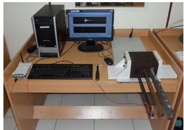
Figure 3: Experimental setup for modal analysis
