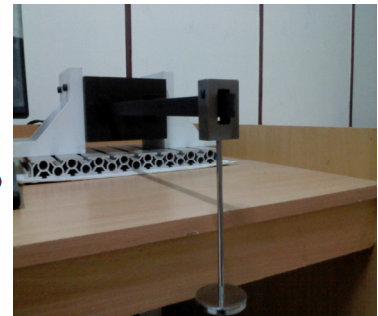
Figure 2. Experimental setup for measuring stiffness
