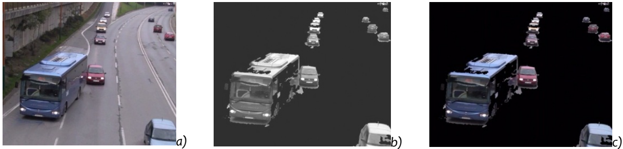
Figure 5: The progress of differential objects creation within the transmitted frames a) Basic frame), b) Differential frame (objects identification), c) Differential objects (transmission itself)
