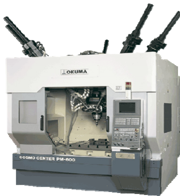
Figure 15. Parallel mechanism machine tool COSMO CENTER PM-600 [53]
