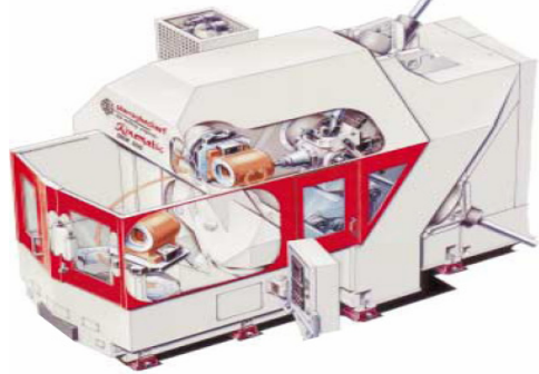
Figure 12. Parallel kinematic machining center SKM 400 (Source Starragheckert)
