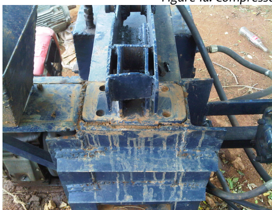
Figure 1b: Compression by lowering the top ram completely into the moulding chamber
