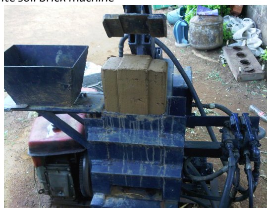
Figure 1c: Ejection of molded brick
