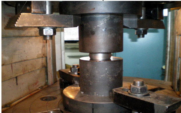
Figure 4. Experimental compression of bimetallic specimen [2.]
