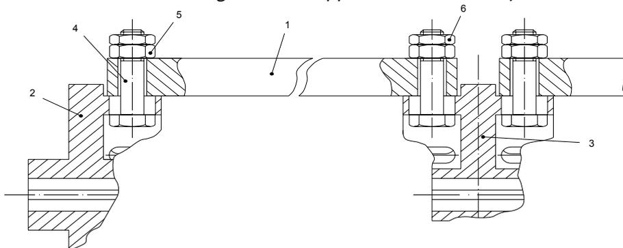
Figure 5. Construction design for experimental samples fixing on intermediate and sideward supporting disks
