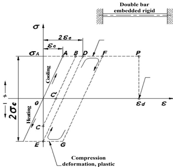
Figure 1. Idealized model of thermal cycles for modeling thermal fatigue
