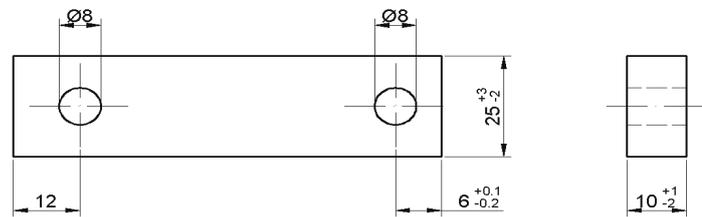
Figure 4. Construction design of a testing sample
