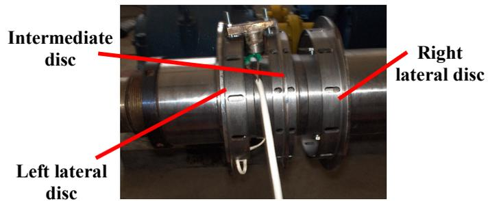
Figure 8. Assembly of samples in which a thermocouple is mounted
