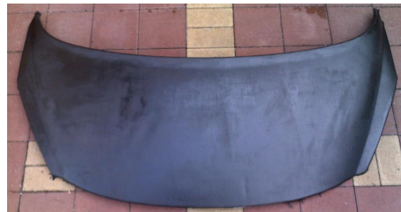
Fig. 9: Hood of the Peugeot 207 made of the carbon composite
