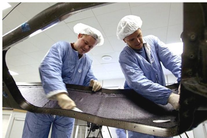
Fig.2: Production of carbon fiber body shell in Renault plant.
