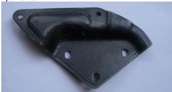
Fig. 8: Part of the bonnet hinge made of carbon composite
